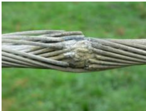
Severe corrosion bulge at 'grease holiday'
