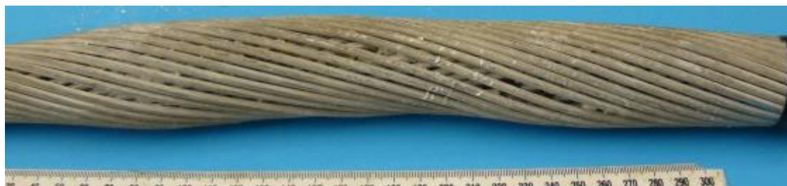
Figure 4: Close-up of bulge 1 (the right-hand bulge of the previous photo)
