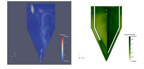
Figure: (Left) Flow velocity of original large tank. (Right) New design of large tank, with water and air supplied at the bottom
